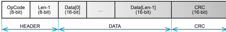
Figure 3-22 maxon serial protocol V1 vs. V2 | maxon serial V1 protocol – Frame structure
